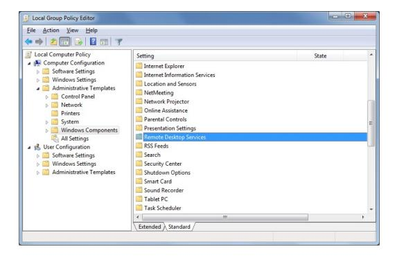
• Then, click on the Remote Desktop Connection Client folder, double-click on the "Allow .rdp files from unknown publishers" setting and enable it, as well as the "Configure server authentication for client":
